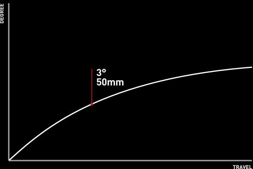
To understand the influence of the engagement angle on the pedal kickback, you need to know how much the freewheel would turn. To do this, one multiplies the pedal kickback by the gear ratio.
