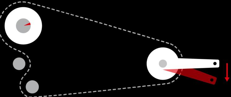
BACKLASH =  $2 \times \prod x$  crank length  $x = \frac{\text{engagement angle}}{360} \times \frac{\text{sprocket}}{\text{chainring}}$
