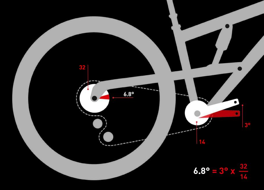
In a system without any POEs, the freewheel body could rotate freely by the appropriate angle in any position, and there would never be any pedal kickback. In a system with infinite POEs or with a high amount of POEs, there is a high probability of pedal kick-back.
